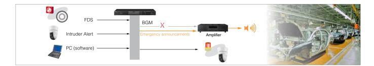
R.E.M. (Recording Endless Message) function enabling operators to create/initiate repeated play back of emergency announcements quickly and evacuate with other occupants before anticipated emergencies such as tsunami
