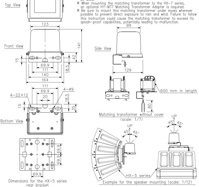
(\*1) When installed under eaves, mount the MT—200 in either way that the tilt angle of its top surface is kept within 45° from the vertical axis. Exceeding this angle will deteriorate the speaker's splash—proof capability.
